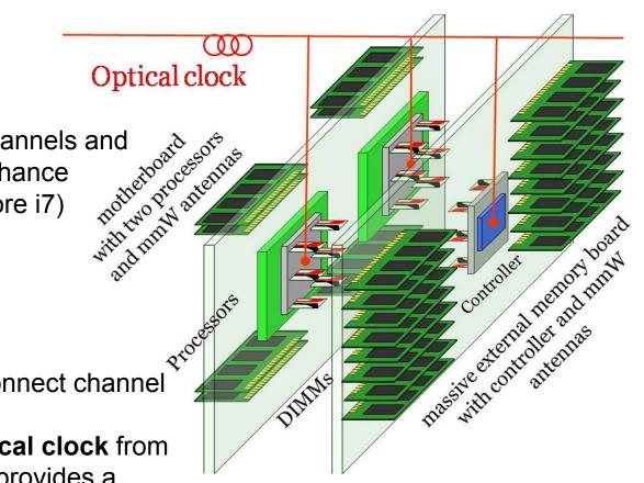
More memory interconnect channels and faster memory DIMMs can enhance system performance. (Intel Core i7)
